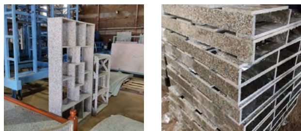
Figure 17. Building materials recycled from liquid packaging board [© AHK E.A. Ltd.]
