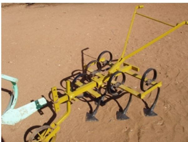
The Nuba hoes manufactured under the UNIDO project have proved suitable for all three types of soil: sandy; sandy loam and clay. They are more environment friendly as they reduce soil erosion by only disturbing the top soil sufficiently for seed planting. They are also lighter than the earlier Nuba hoes and therefore more easily operated by women and more transportable.
