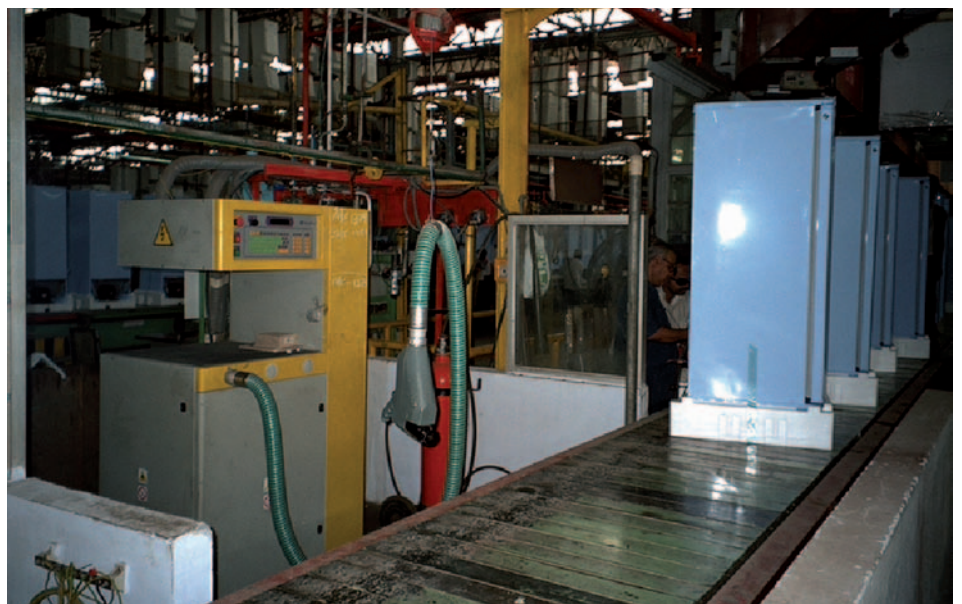
Production line for charging of refrigerants
