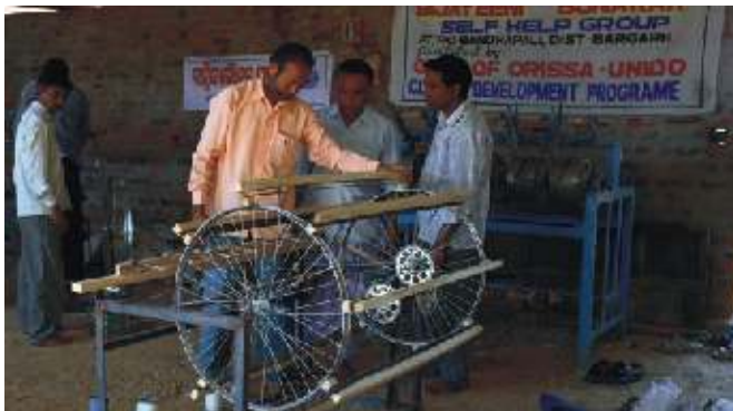
Auto weft winding machine with gear and brake
