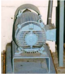
15 kW Motor Efficiency is ~ 91%
