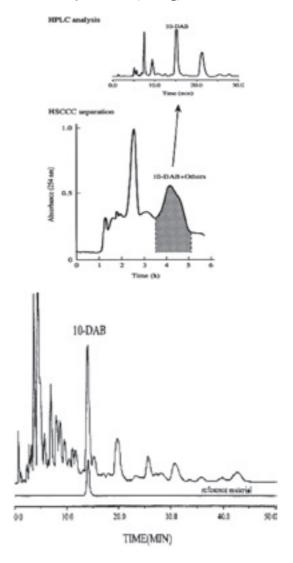
Figure 11: Separation and purification of 10-deacetylbaccatin III (DAB) by HSCCC
