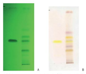
Figure 1: TLC chromatograms as visualized (A) under 254 nm UV and (B) after being sprayed with anisaldehyde-sulphuric acid reagent
