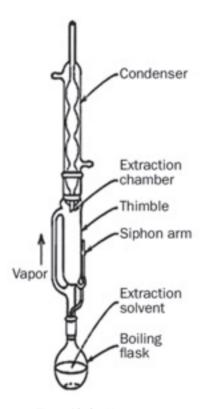
Figure 10: Soxhlet extractor
