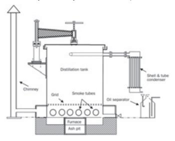
Figure 3: CIMAP's improved field distillation unit
