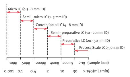
Figure 1: Classification of HPLC according to column diameter
