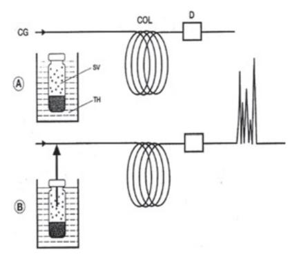
Figure 3: Static headspace trapping technique
