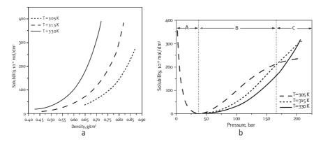
Figure 2: Solubility of 1,4-bis-(n-propylamino)-9,10-anthraquinone in supercritical CO<sub>2</sub>: as a function of solvent density (2a) and of pressure (2b)
