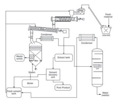
Figure 2: Flowsheet of microwave-assisted extraction (courtesy, Radient Technologies Inc).
