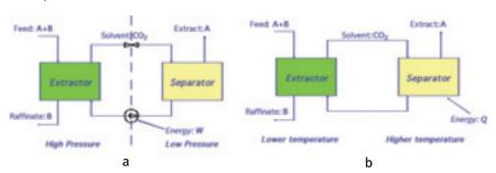
Figure 3: Block flow diagrams of simple SFE processes: with separation obtained by pressure change (a) and by temperature change (b)
