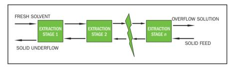
Figure 2: Multistage counter-current solid-liquid extraction
