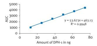
Figure 2: Calibration curve of DPH-1
