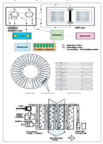
Figure 9: Centrifugal partition chromatography setup
