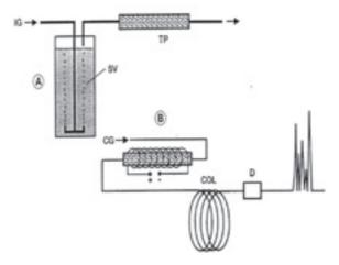
Figure 4: Dynamic headspace trapping technique
