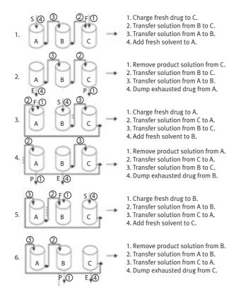
Arrows indicate transfer of material to or from the vessels. An asterisk(.) is added after each contact stage. Key: F = fresh drug. S = solvent. P = product. E = exhausted drug. A, B, C, extraction vessels. Start with C empty and units A and B containing drug, with A more nearly exhausted.
