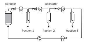
Figure 4: Single extractor, multiple separator scheme
