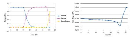
Figure 5: a) Fractional composition versus time, and b) Energy consumption versus time for the total fractionation case
