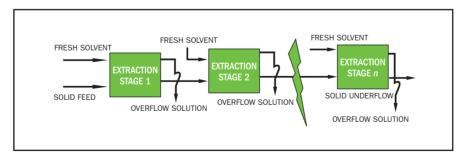
Figure 3: Multistage co-current solid-liquid extraction
