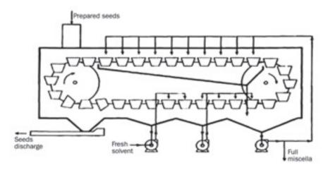
Figure 5: Continuous horizontal extractor
