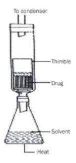
Figure 5: Apparatus for the continuous extraction of drugs
