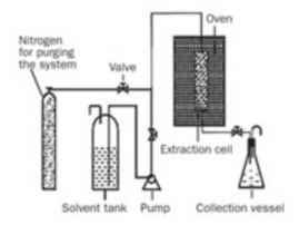
Figure 11: Accelerated solvent extraction
