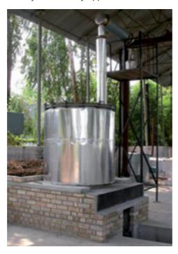
Figure 5: Distillation unit with cohobation
