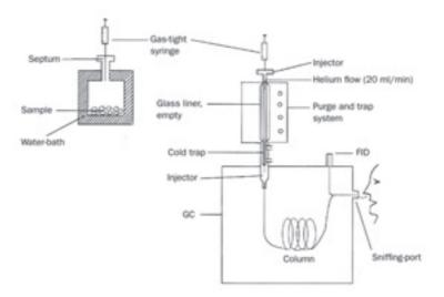
Figure 5: Static headspace trapping technique
