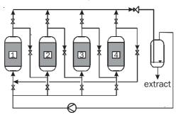
Figure 5: Multiple extractor, single separator scheme
