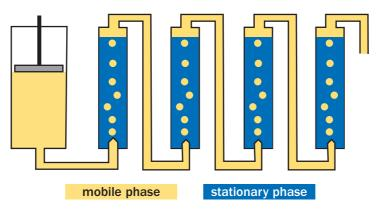
Figure 3: Droplet counter-current chromatography
