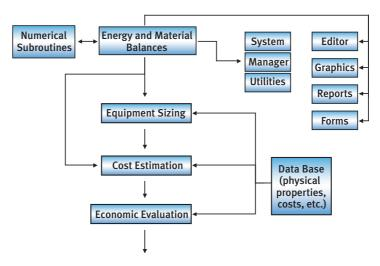
Figure 2: General scheme of a steady-state process simulator
