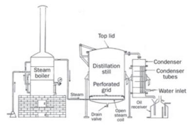
Figure 4: Boiler-operated steam distillation unit
