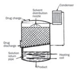
Figure 6: Continuous extraction: large-scale plant
