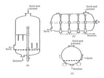
Figure 4: Pot extractor and rotating extractor
