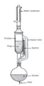
Figure 4: Soxhlet apparatus for hot extraction
