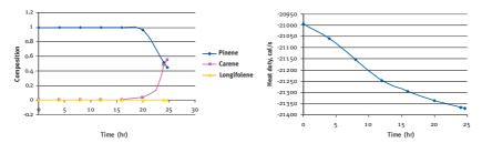
Figure 3: a) Fractional composition versus time, and b) Energy consumption versus time for the base case
