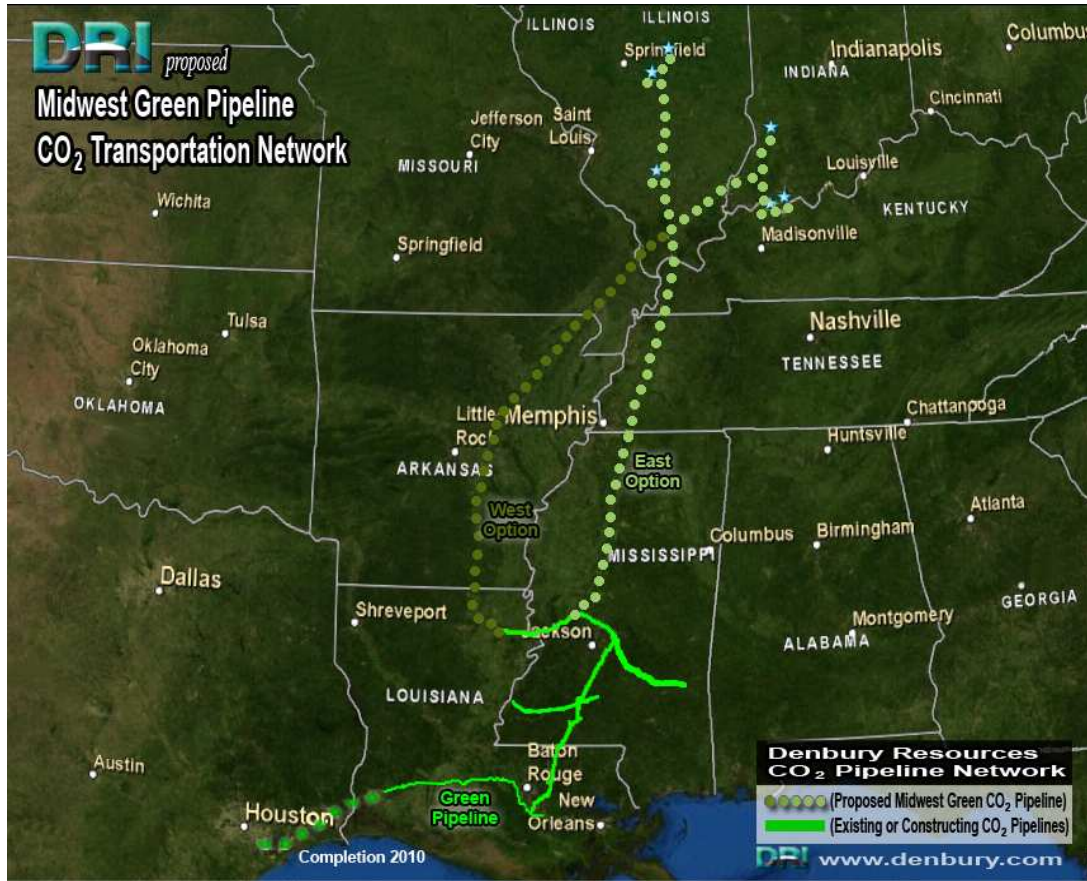
Figure 7. Denbury Resources' Strategic Vision for Moving Midwest CO 2 Supplies to the U.S. Gulf Coast CO 2 -EOR Market
