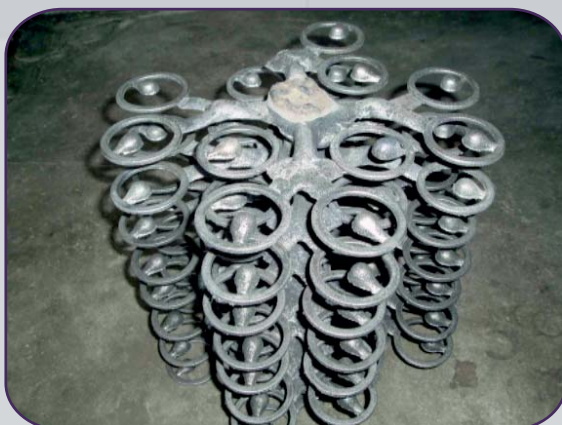
By modifying Gate and runner, rejection reduced by 30 %
