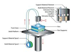
Fused deposition modeling (FDM)—This process uses hot nozzles to extrude polymeric material into position, using one nozzle to extrude support material and a second to extrude the part.
