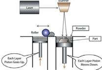
**Powder bed (laser) sintering**—Laser sintering fuses together powder from a bed. Originally, laser sintering could produce polymer as well as metallic and ceramic parts (using each type of powder), with binders needed in the case of metal or ceramic powders. Recently, more powerful lasers have been used to directly sinter metal and ceramic without the use of binders (Hopkinson 2010).
