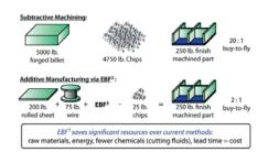
**Electron beam melting or e-beam melting (EBM)**—This is a process that uses an electron beam in place of a laser to directly melt metal powder into parts. (Arcam, a Swedish manufacturer, has pioneered the use of electron beam melting (Taminger 2008).)
