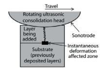
**Ultrasonic consolidation (UC)**— One of the newest additive manufacturing technologies, patented by an American company called Solidica and in development by Solidica and the Edison Welding Institute (Slattery 2011). This process uses metal foils held together under pressure, combined with ultrasonic vibrations that create a weld between layers of foil, which are then machined to the desired shape (Domack and Baughman 2005).
