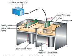
Inkjet Deposition (3D Printing)—This process uses an inkjet similar to those found in 2D printers. It works by depositing a binder on a powder bed that joins the powder in each layer without the use of lasers.
