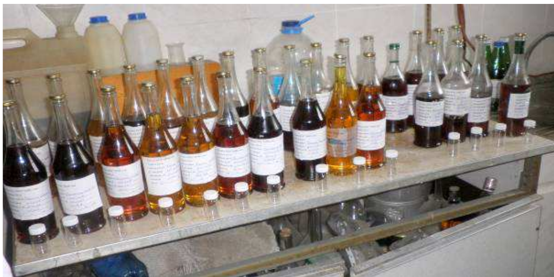
Picture 1. Some samples of oil to check their PCB content at the laboratory of MENR.
