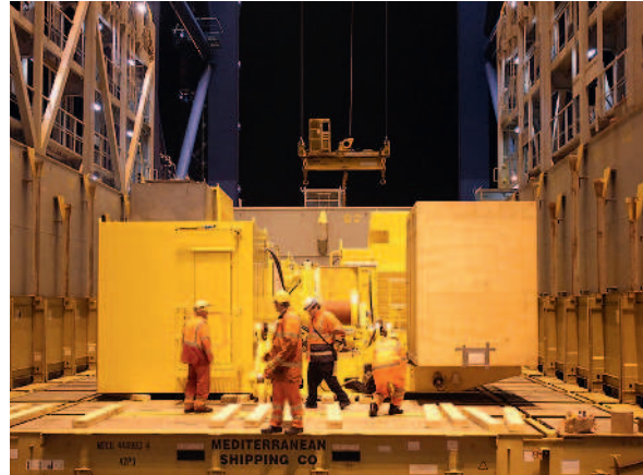
Handling oversized or "out-of-gauge" cargo on board an MSC-owned containership.
