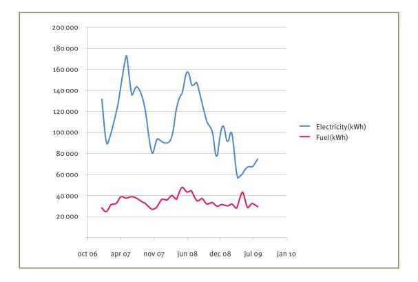
Figure VI shows the trend of monthly energy use of a factory. It seems to indicate a seasonal effect and a baseload in each energy use, i.e. about 60,000 kWh for electricity and 25,000 kWh for fuel use. In this case fuel use is shown in kWh. Some organizations do this to allow clear comparison while others use GJ.
