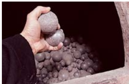
Rocks are crushed manually using hammers (not shown), and then milled using ball mills (Tanzania, 2010).
