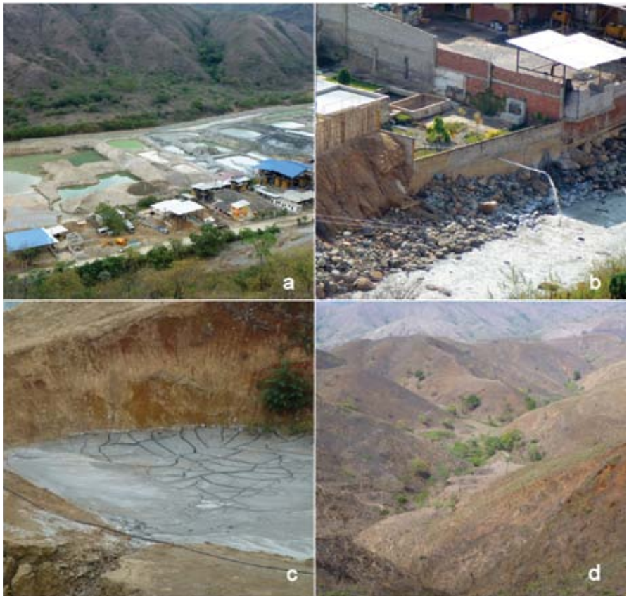
Poorly managed waste, contaminated sites, and a solution for artisanal and small scale gold mining in Portovelo, Ecuador: (a) substandard tailings ponds; (b) direct discharge to rivers; (c) site contaminated with tailings; (d) an adjacent valley (burned pasture) that is a suitable for a tailings impoundment that meets international standards and that can serve the needs of the ASGM community.
