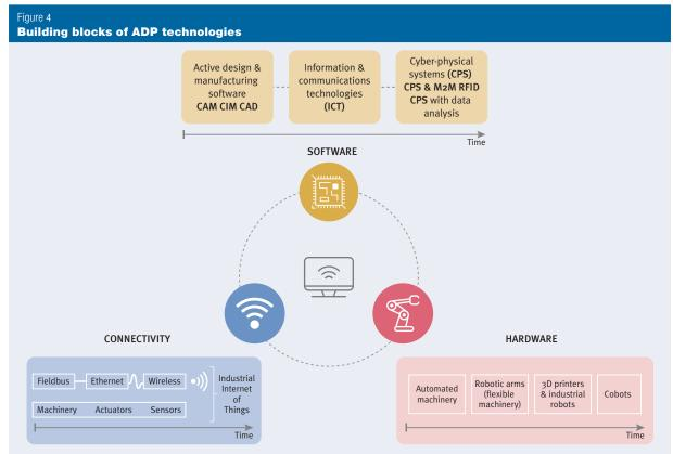
Note: CAM is computer-aided manufacturing, CAD is computer-aided design, CIM is computer-integrated manufacturing, M2M is machine to machine, and RFID is radio-frequency identification. CIM links CAD, CAM, industrial robotics, and machine manufacturing through unattended processing workstations. Source: Andreoni and Anzolin 2019.
