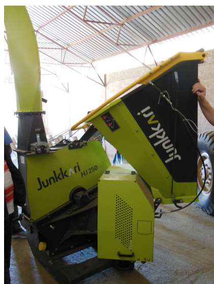
Figure 5.5 - Junkkari HJ 250 GT chipper, imported from Finland and in use at UNAM, Neudamm Campus (20 km east of Windhoek) and wood chips measuring an average 3 cm x 7 cm in size
