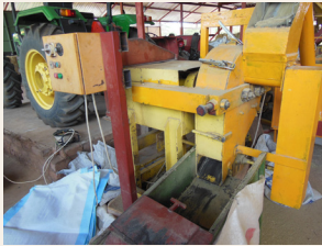
Figure 5.13 - Pelletizing machine at BosPro Products and, 50-kg size bags filled with freshly made pellets
