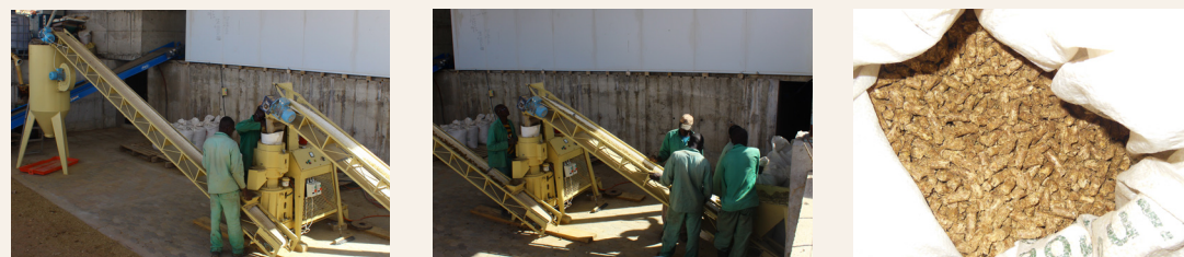
Figure 5.9 - Pelletizing line at Langbeen Farm with a sample of the pellets (the size of the pellets is 8 mm)
