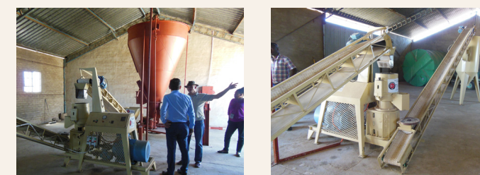
Figure 5.12 - Pelletizing production line at the UNAM-Neudamm Campus
