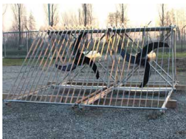
Figure 3. Smart Free Stream canal turbine
