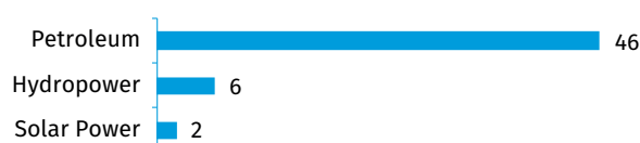
Figure 1. Annual Electricity Generation by Source in Saint Vincent and the Grenadines in 2020 (GWh)
