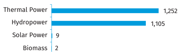
Figure 2. Annual Electricity Generation by Source in Suriname in 2020 (GWh)
